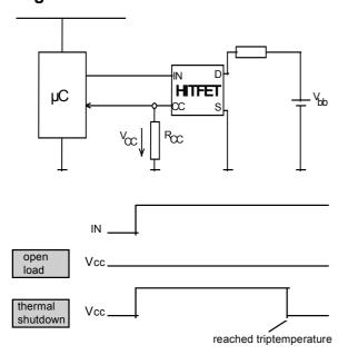
The accuray of Vcc is at each temperature about  $\pm 10~\%$
