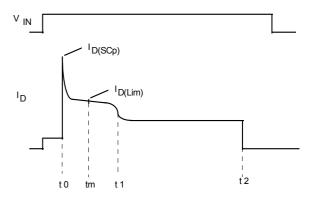
t<sub>0</sub>: Turn on into a short circuit
