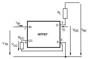
The ground lead impedance of  $R_{\rm CC}$  should be as low as possible
