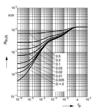
**Permissible Puls Load**  $R_{\text{thJS}} = f(t_p)$ BCR135W
