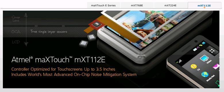
The Atmel maXTouch mXT112E mutual capacitance touchscreen controller is suitable for use in a wide range of devices ranging digital cameras to personal navigation devices and feature phones. The highly responsive IC can interpret up to four touches on the touchscreen whilst avoiding the "ghosting" problems of self-capacitance solutions.
