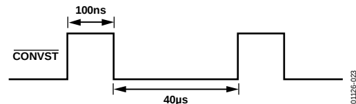
Figure 21. \overline{\text{CONVST}} When Temperature Channel Selected
