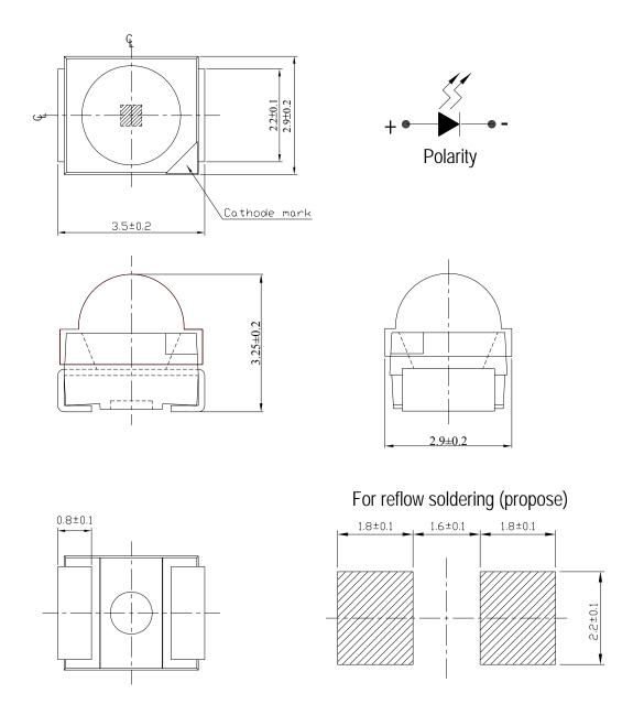
**Note:** Tolerances Unless Dimension ±0.1mm, Unit = mm
