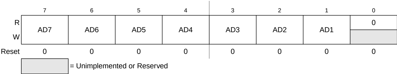
Figure 10-3. IIC Address Register (IICA)
