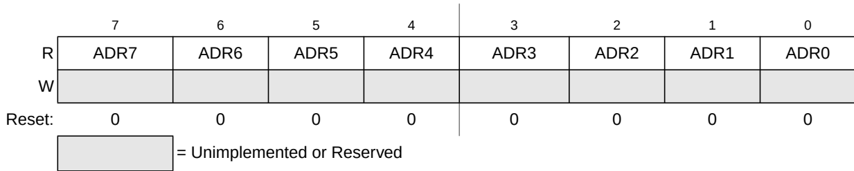
Figure 9-6. Data Result Low Register (ADCRL)
