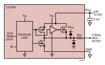
Figure 14. Digital Output Buffer
