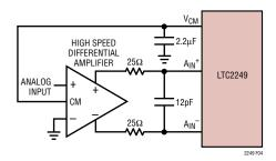
Figure 4. Differential Drive with an Amplifier
