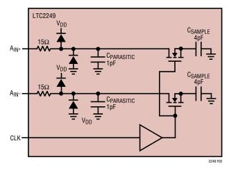
Figure 2. Equivalent Input Circuit
