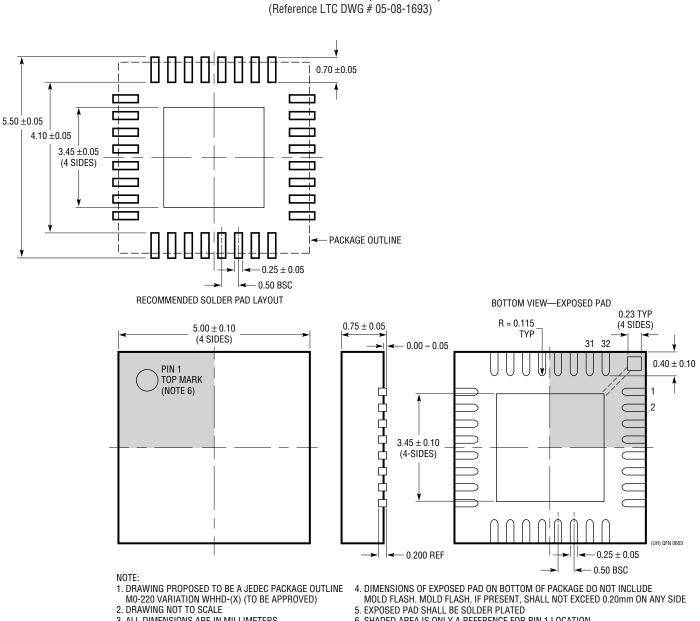
UH Package 32-Lead Plastic QFN (5mm  $\times$  5mm)
