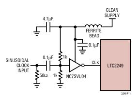
Figure 11. Sinusoidal Single-Ended CLK Drive
