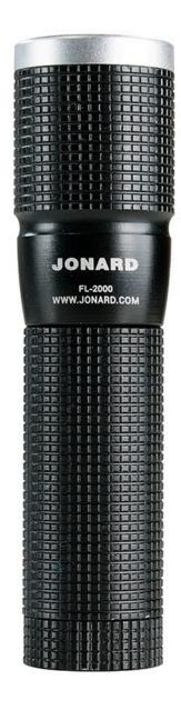
A high quality LED Flashlight powered by a single AA alkaline battery. Housing is rugged aluminum suspended from a clip-on lanyard. Brightness is 120 lumens and the beam is adjustable to meet the working environment. Zoom in for a tight narrow beam and zoom out for a wide light. Hold the head of the flashlight with one hand and the body with the other. Simple in and out movement adjusts the light. Simple push-button operation.
