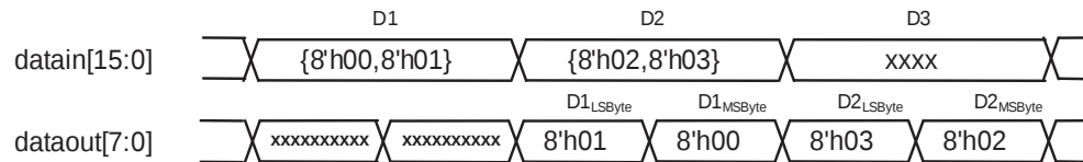
Figure 2–5. Byte Serializer Operation (Note 1)
