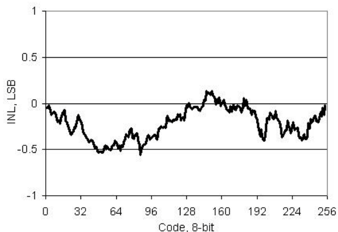
Figure 11-34. IDAC INL vs Input Code, Range = 255 \mu A, Sink Mode
