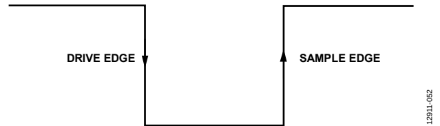
Figure 42. SPI Mode 3 SCLK Edges
