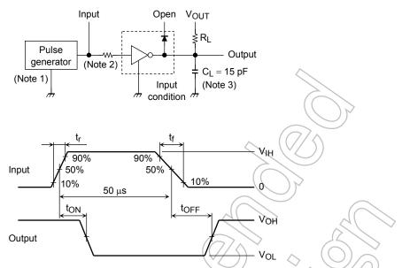
Note 1: Pulse width 50  $\mu$ s, duty cycle 10% Output impedance 50  $\Omega$ ,  $t_r \le 5$  ns,  $t_f \le 10$  ns
