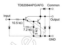
Note: The input and output parasitic diodes cannot be used as clamp diodes.
