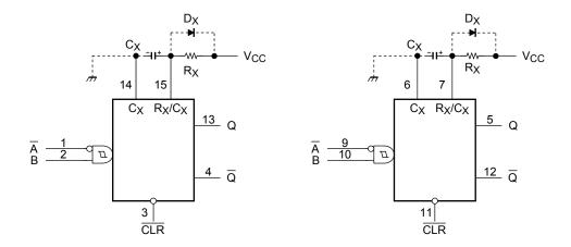
Note 1: C<sub>X</sub>, R<sub>X</sub>, D<sub>X</sub> are external capacitor, resistor, and diode, respectively.
