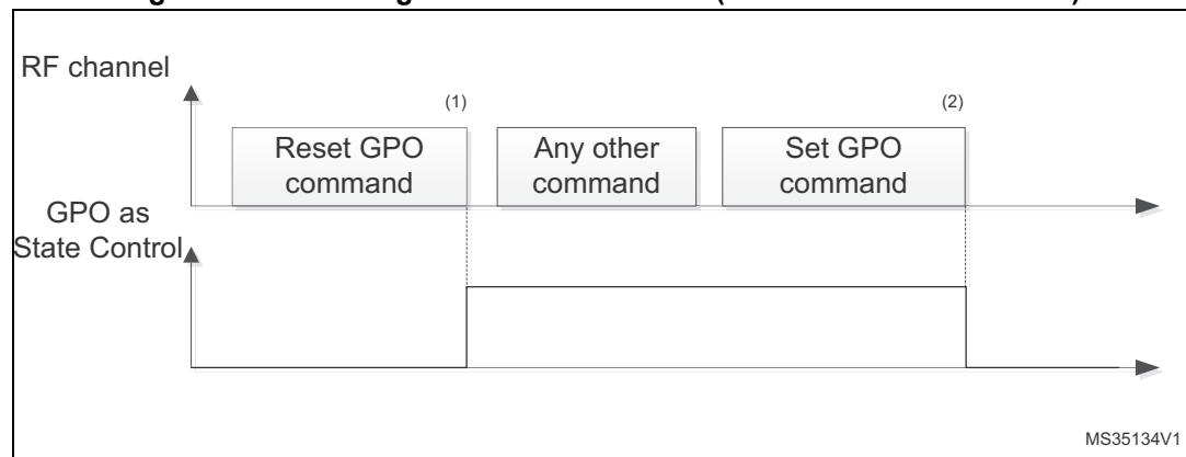
Figure 9. GPO configured as State Control (GPO field = 0x50 or 0xD0)
