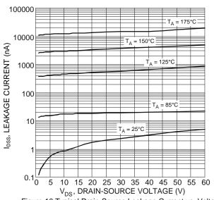
Figure 10 Typical Drain-Source Leakage Current vs. Voltage
