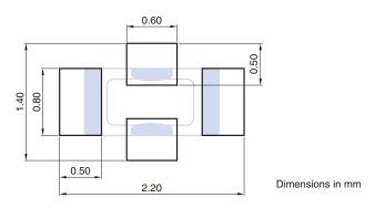
Line width be designed to match  $50\Omega$  characteristic impedance depending on PCB material and thickness.
