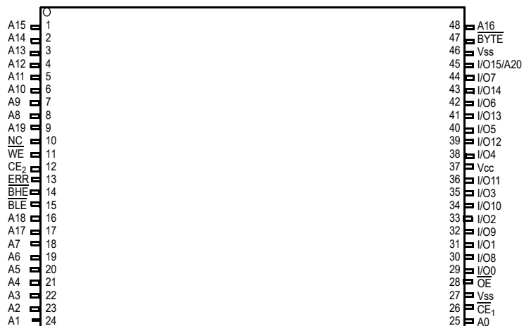
Figure 5. 48-pin TSOP I Pinout (Dual Chip Enable with ERR) – CY62167GE [9, 10]
