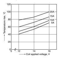
1.-(2) Coil temperature rise (85°C 185°F) Sample: CP1-12V, 6pcs Point measured: Inside the coil
