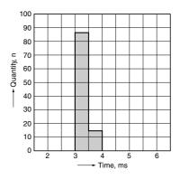
6. Distribution of release (reset) time Sample: CP1-12V, 100pcs Ambient temperature: 20°C 68°F
