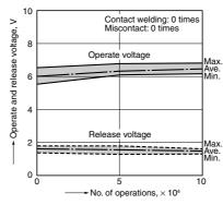
7.-(2) Electrical life test for wiper load (motor free)
