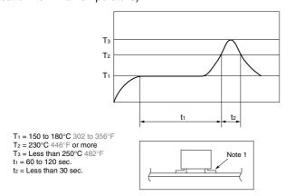
Temperature profile indicates the temperature of the soldered part (Note 1) of terminals on the surface of the PC board, however, for other areas such as the surface of relay case, make a setting so that you do not exceed the recommended conditions.
