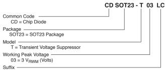
LC = Low Capacitance Diode
