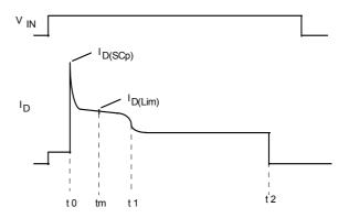
t<sub>0</sub>: Turn on into a short circuit
