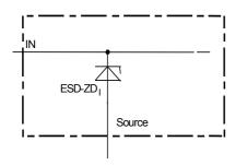
ESD zener diodes are not designed for DC current > 2 mA @  $V_{\text{IN}}$ >10V.
