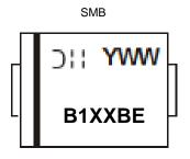
B1XXBE = Product Type Marking Code, ex: B150BE DII = Manufacturers' Marking YWW = Date Code Marking Y = Last Digit of Year (ex: 0 for 2020) WW = Week Code (01 to 53)
