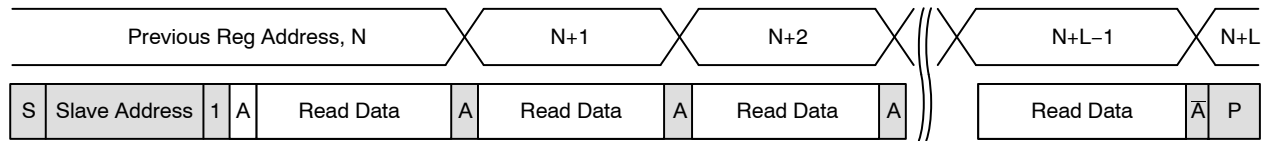
Figure 45. Sequential READ, Start from Current Location
