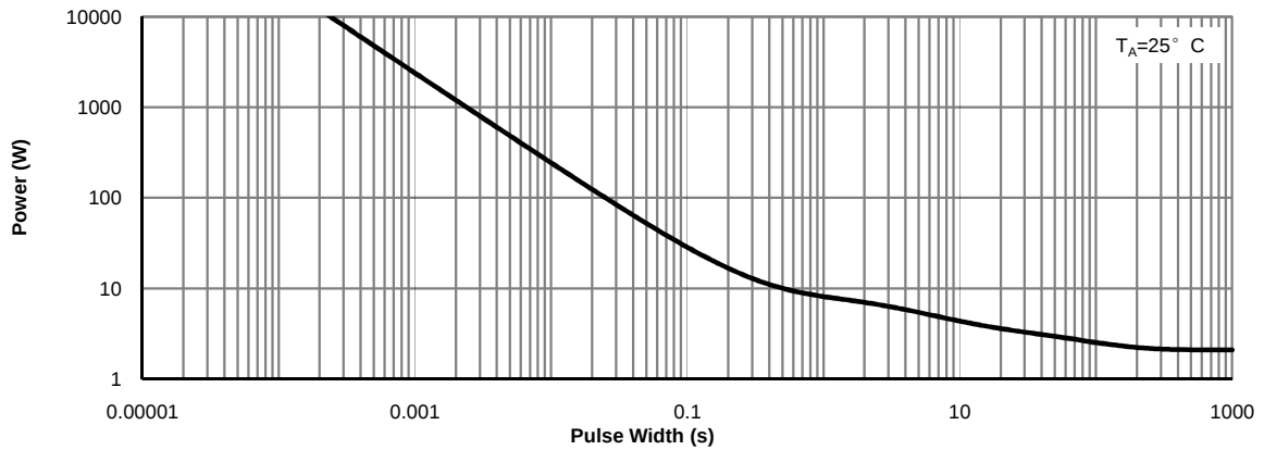
Figure 14: Single Pulse Power Rating Junction-to-Ambient (Note H)
