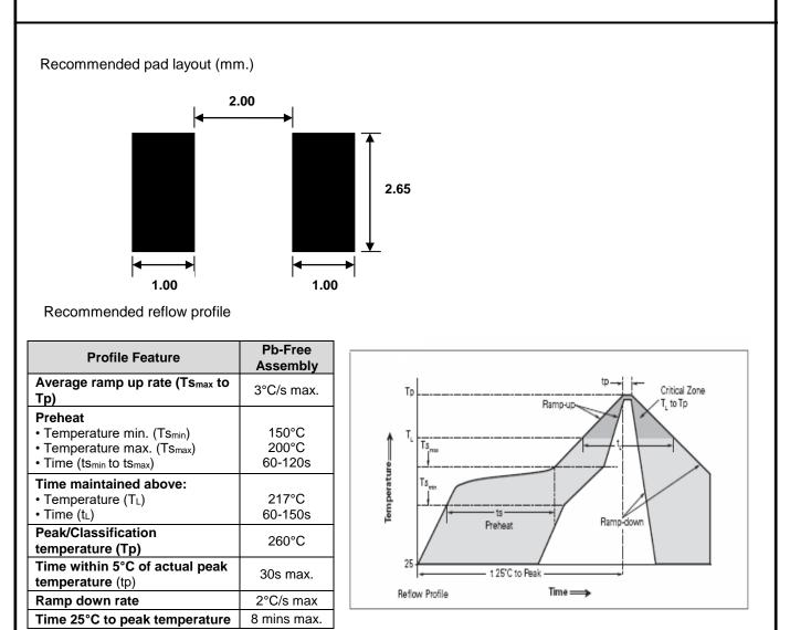
Note: All temperatures refer to top side of the package, measured on the package body surface.
