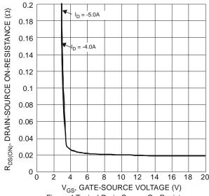
Figure 4 Typical Drain-Source On-Resistance vs. Gate-Source Voltage
