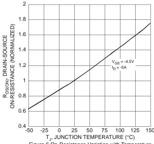
Figure 6 On-Resistance Variation with Temperature
