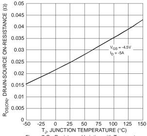
Figure 7 On-Resistance Variation with Temperature
