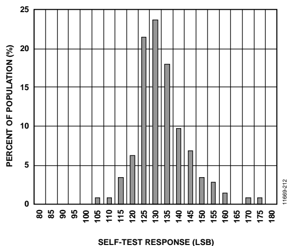
Figure 16. Z-Axis Self-Test Response at 25°C, V_S = 2.5\text{ V}
