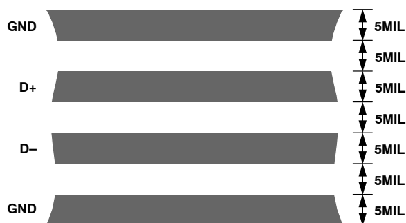
Figure 34. Typical Arrangement of Signal Tracks
