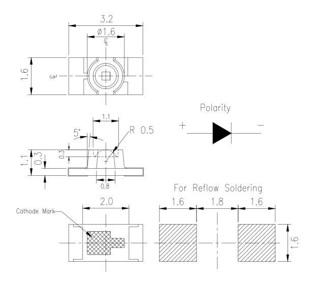
**Note:** The tolerances unless mentioned is  $\pm 0.1$  mm , Angle $\pm 0.5^{\circ}$ , Unit = mm
