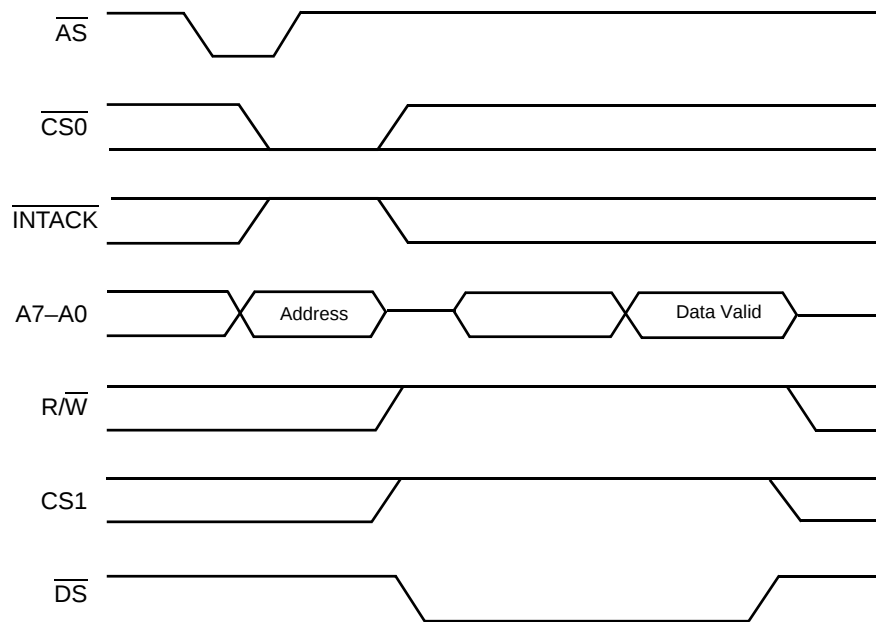
Figure 18. Z80230 Read Cycle Timing
