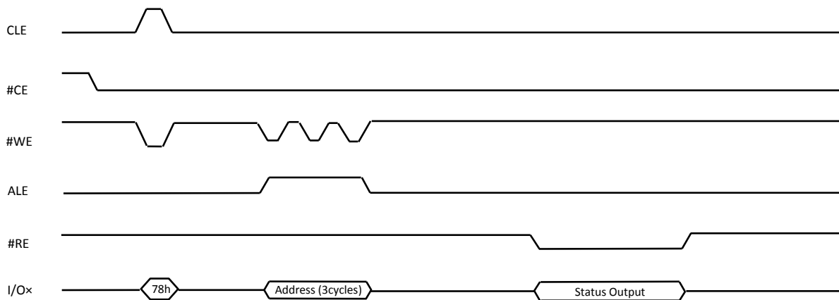
Figure 9-10 Read Status Enhanced (78h) Operation
