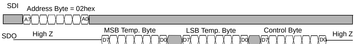
FIGURE 4-3: Serial Interface Timing Diagrams (CP=0).
