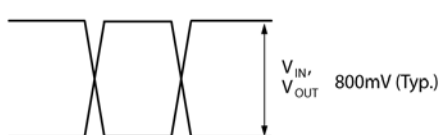
Figure 1a. Single-Ended Voltage Swing
