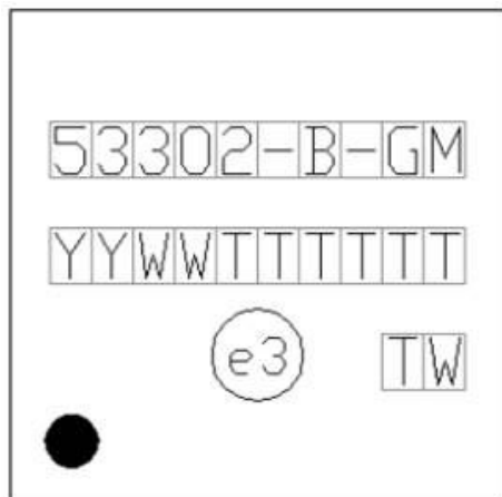
Figure 8.4. Si53302 Top Marking
