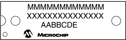
28-Lead PDIP (Skinny DIP)
