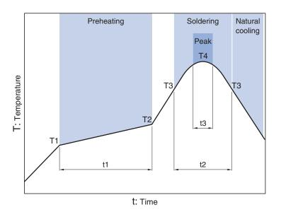
Preheating Soldering Peak Temp. Time Temp. Time Temp. Time Τ1 T2 t1 тз t2 Т4 t3 150°C 180°C 90 to 120s 230°C 40s 255°C 10s max.
