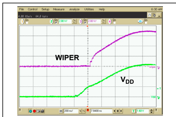
FIGURE 2-15: 2.1 k \Omega – Power-Up Wiper Response Time.
