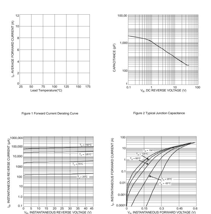
Figure 3 Typical Reverse Characteristics
