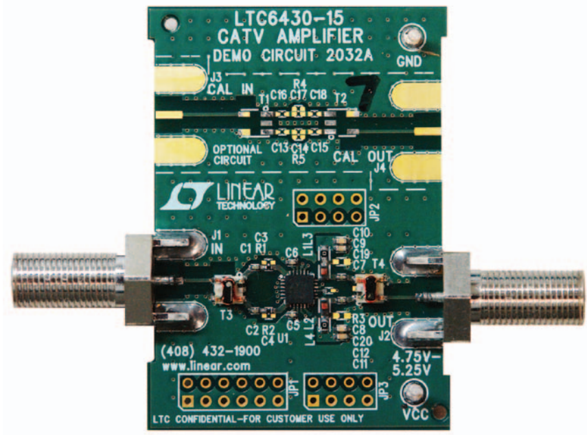
Figure 17. LTC6430-15 CATV Evaluation Board
