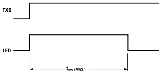
Figure 4. TXD "stuck on" protection waveform.
