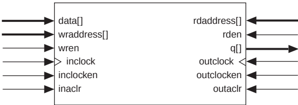
Figure 2–13. Simple Dual-Port & Single-Port Memory Configurations
