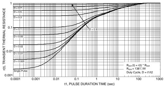
Figure 13 Transient Thermal Resistance
