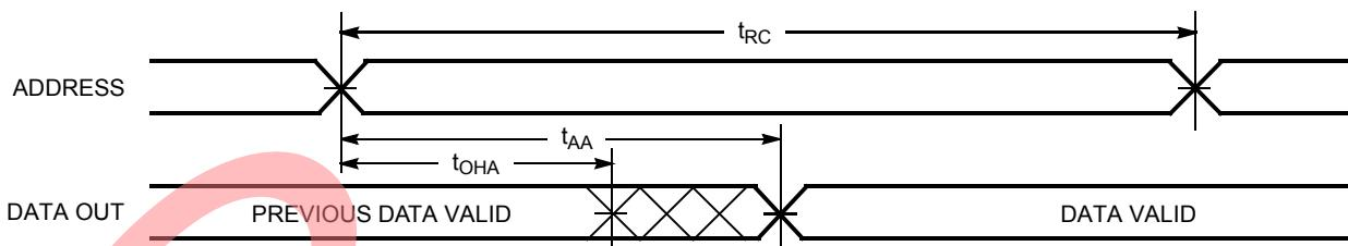
Read Cycle No. 2 ( $\overline{OE}$  Controlled)<sup>[13, 14]</sup>
