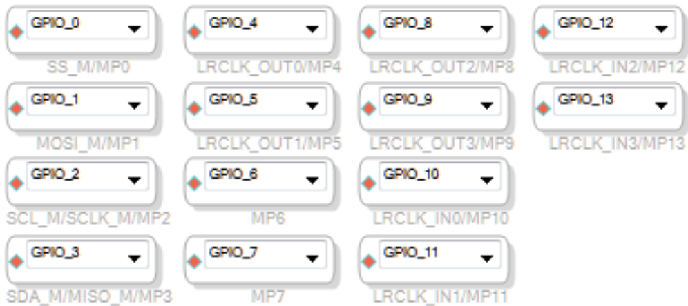
Figure 76. Complete Set of General-Purpose Outputs in SigmaStudio
