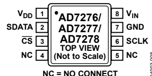
Figure 9. 8-Lead MSOP Pin Configuration
