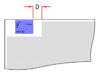
Additional ground and components near the antenna should be at a distance of at least 2 mm. Where possible the antenna should be clear of ground from both sides, although the antenna can work well with a minimum clearance of  $D \ge 2$  mm as shown in the drawing above.
