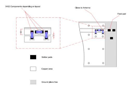
The antenna feed pad is indicated in the drawing above. Additional pads are for mechanical attachment only and should not be grounded.
