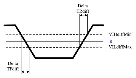
**AC and DC Output Measurement Levels**
