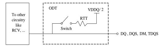
The switch is enabled by the internal ODT control logic, which uses the external ODT pin and other control information. The value of RTT is determined by the settings of Mode Register bits. The ODT pin will be ignored if the Mode Register MR1 and MR2 are programmed to disable ODT and in self-refresh mode.
