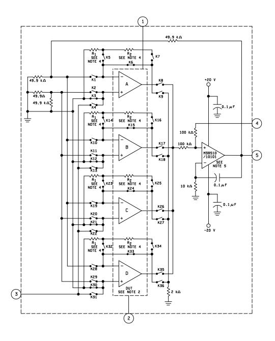
FIGURE 3. Test circuit for channel separation.
