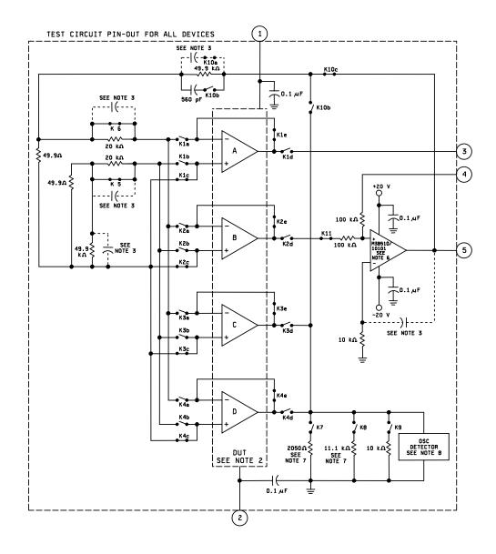
FIGURE 2. Test circuit for static tests.
