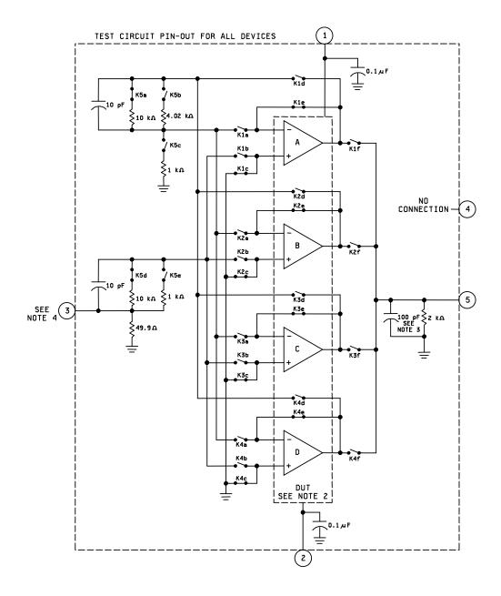
FIGURE 4. Test circuit and waveform for transient response .
