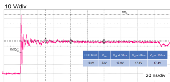
Figure 7: ESD response to IEC 61000-4-2 (+8kV contact discharge)
