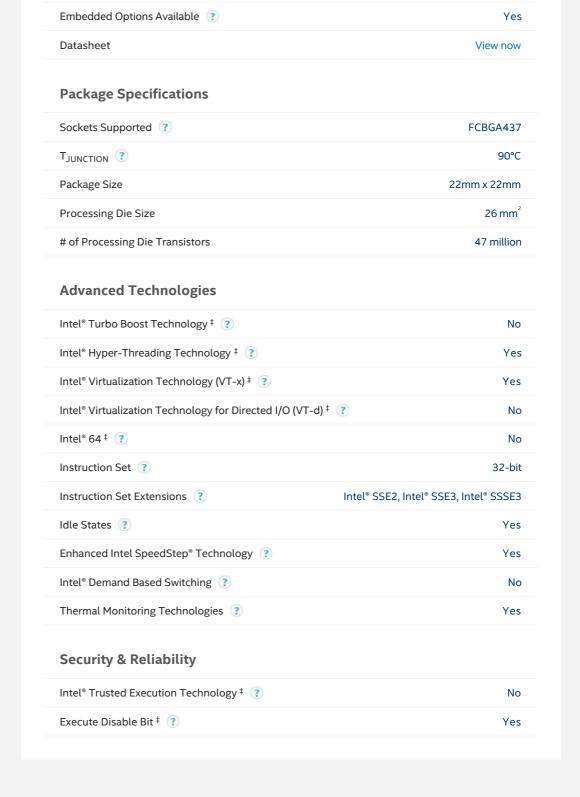
More support options for Intel Atom® Processor Z530P (512K Cache, 1.60 GHz, 533 MHz FSB)
