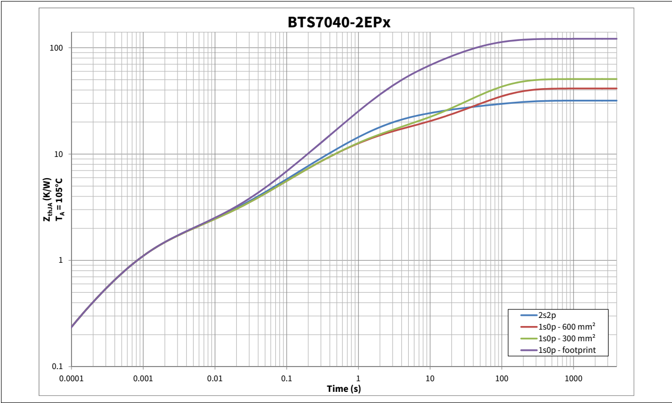
Figure 9 Typical Thermal Impedance. PCB setup according Chapter 4.4.1
